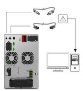
Both RS232 and USB connections allow for 2 way communication between the device connected and the UPS. This can be used for both issuing configuration commands, communicating with the UPS and issuing shutdown commands. When connected via USB to a PC the UPS will present itself as a HID compliant ACPI device allowing for zero configuration shutdown initiated by the UPS in the event of a power failure.
